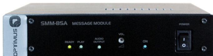
Module for sending up to 58 audio message sequences MP3 / OGG / WAV to the PA system, 50 with time schedule and 8 with remote program activation. Messages can combine 1, 2 or 3 different audio files.
